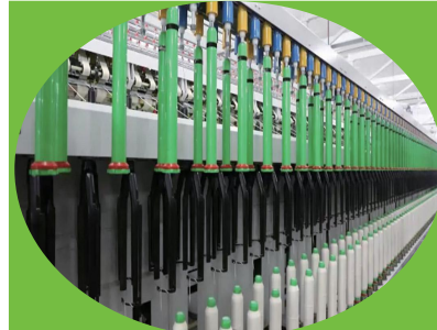
Automatic doffing of roving
